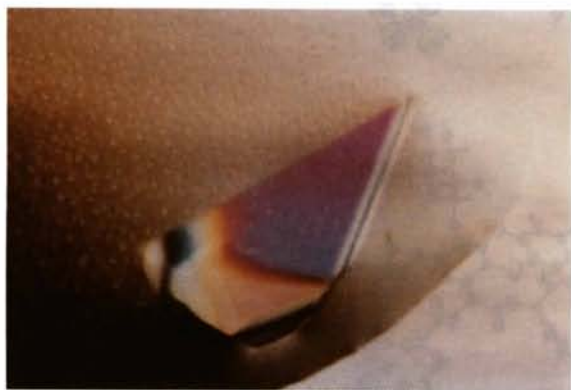
Fig. 3. Picture of a single crystal of balhimycin. This crystal was grown by Dr Bob Cudney under similar conditions to those employed for the crystal used for data collection; we are grateful to him for providing this photograph.
